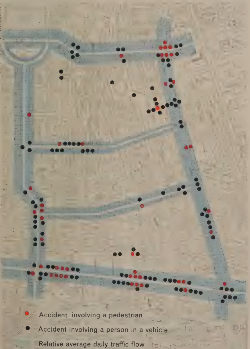
173 The record of accidents in the study area from July-December, 1962 and the relative average daily flow of traffic. (The present one-way traffic system in Tottenham Court Road was introduced in 1961.)
